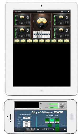
The tablet and plantwide wireless network enables operators to take advantage of SCADA HMI dashboards remotely.
